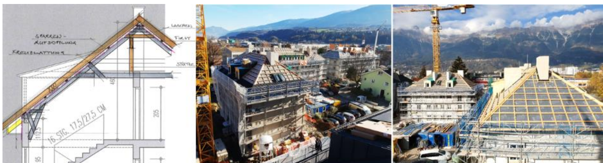
FIGURE 21: IN 22 & 23: COLD ATTIC INTO THE THERMAL SHELL
