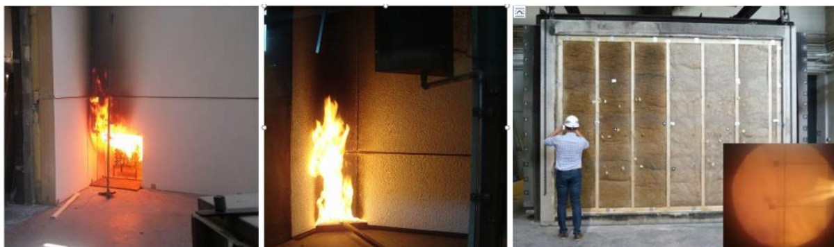
FIGURE 45: FIRE BEHAVIOUR AND FIRE RESISTANCE TESTS TO PROOF THE FIRE SAFETY OF PREFABRICATED FACADE ELEMENTS [4, 5] © BADERGRUBER, T.; LE LEVÉ, C.
